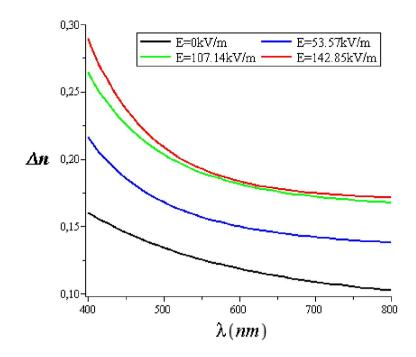
Fig. 2 Birefringence of MBBA LC vs. wavelength.
