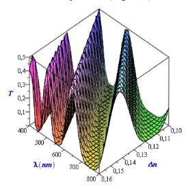
Fig. 2 Transmission factor of the Wood filter with 2 elements (MBBA LC) vs. wavelength vs. birefringence.
