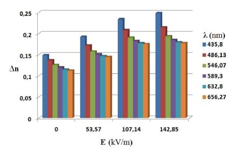
Fig. 1 Birefringence of MBBA LC vs. intensity of the electric field.
