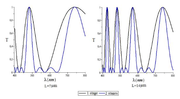
Fig. 4 Transmission factor of the Lyot filter vs. wavelength.
