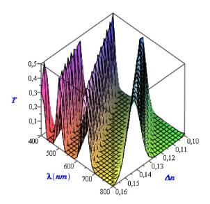
Fig. 3 Transmission factor of the Wood filter with 5 elements (MBBA LC) vs. wavelength vs. birefringence.
