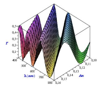
Fig. 1 Transmission factor of the Wood filter with MBBA LC vs. wavelength vs. birefringence.
